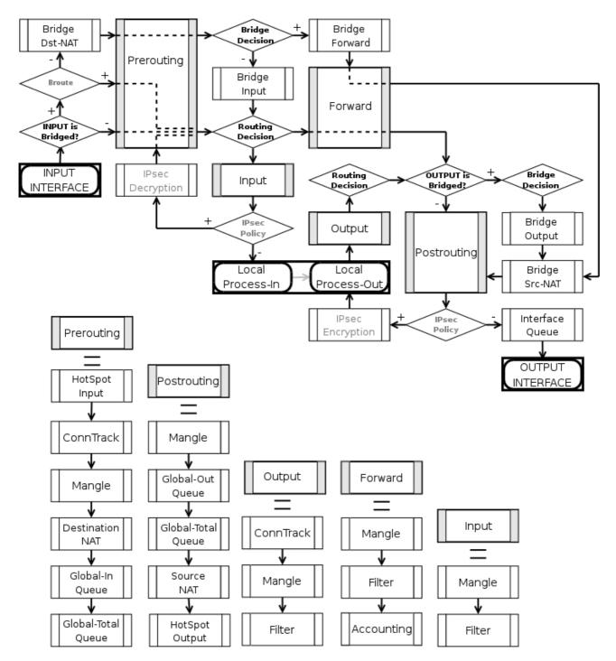
As can be seen on the diagram, there are five chains in the processing pipeline. These are **prerouting**, **input**, **forward**, **output** and **postrouting**. The actions performed on a packet in each chain are discussed later in this chapter.
