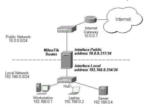
The server'would have been s address now is 192.168.0.4, and we are running web server on it that listens to the TCP port 80. We want to make it accessible from the Internet at address:port 10.0.0.217:80. This can be done by means of Static Network Address translation (NAT) at the MikroTik Router. The Public address:port 10.0.0.217:80 will be translated to the Local address:port 192.168.0.4:80. One destination NAT rule is required for translating the destination address and port:
