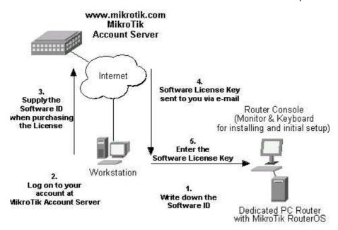
After installing the router and starting it up for the first time you will be given a Software ID.
