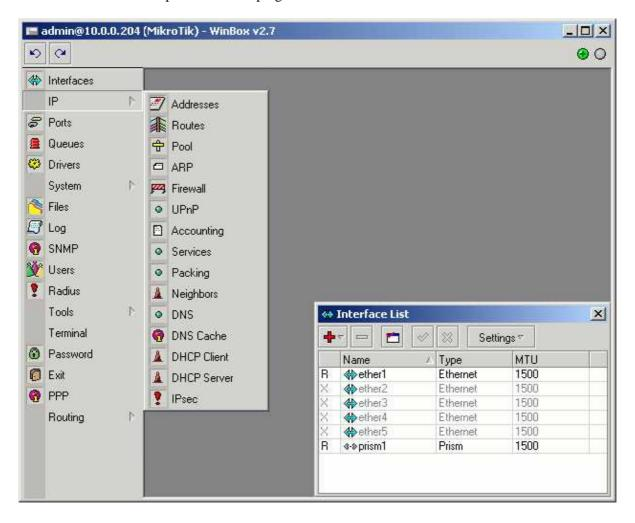
The Winbox Console uses TCP port 3986 (not secure) or 3987 (secure; requires **security** package to be installed). After logging on to the router you can work with the MikroTik router's configuration through the Winbox console and perform the same tasks as using the regular console.
